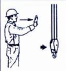
TRAVEL. Extend arm forward, hand open and slightly raised; make pushing motion in direction of travel.
